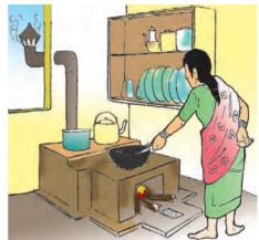
Similarly, the hot smoke from the burning firewood also goes to the second mouth. The food on the second mouth of the oven is cooked with the heat. This way, improved earthern stove saves fuel. The surplus hot air/smoke goes out of the house through the chimney kept ahead of the second mouth.
