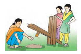
Dhiki has been in use from the very beginning for pounding paddy and for making beaten rice. It is made up of a long log of wood which is about 2 metres in length, 15 cm in breadth and 10 cm thick/high. The tail of a Dhiki is made flat to keep the feet to raise it. At the one third parts from the tail of the log, a wooden bar (Aaglo) is kept crosswise on the pillars on both sides so that the Dhiki is between them. The Dhiki has a pestle on the middle
