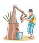
high pressure falls on the sugarcane and the juice comes from them. The juice comes out of the mill through a small hole and collected in a bucket. People make molasses and brown sugar out of the sugarcane juice.
